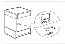
The recommended cross-section area is six square millimetres (6 mm²). When you refit the mains terminal cover, make sure that the lower tabs are located inside the bottom edge of the aperture, before you fix the two screws into the top edge of the mains terminal cover. Make sure that the cover is securely fas-
